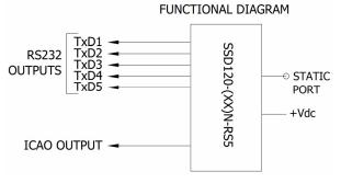
data ports. The SSD120-(XX)N-RS5 provides a simple, robust means of transmitting serial altitude data to multiple aircraft systems.
